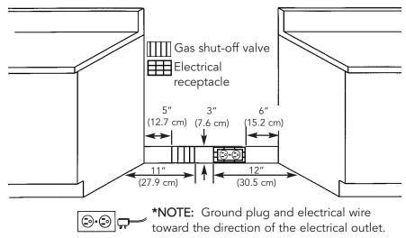
A properly-grounded horizontally- mounted electrical receptacle should be installed no higher than 3" (7.6 cm) above the floor, no less than 6" (15.2 cm) and no more than 12" (30.5 cm) from the right side (facing product). Check all local code requirements.
