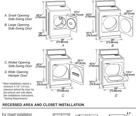
For closet installation with a door, minimum ventilation openings in the top and bottom of the door are required. Louvered doors with equivalent air openings are acceptable.
