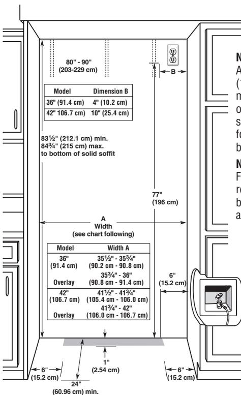
**NOTE:** A clearance of 1/2" (1.3 cm) must be maintained in front of the refrigerator's side trim in order for the top grille to be removed.
