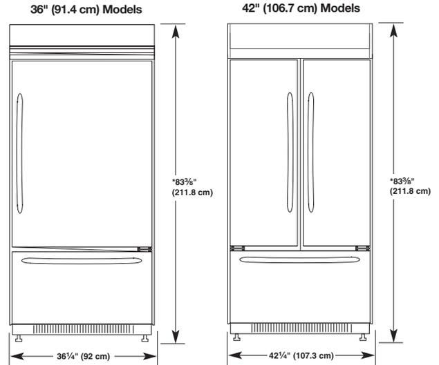
\* When leveling legs are fully extended to 1/4" (3.2 cm) below rollers, add 1 1/8" (2.9 cm) to the height dimensions.
