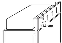
If the anti-tip boards are needed, they must be attached to the rear wall studs 80" to 90" (203 to 229 cm) above the floor.
