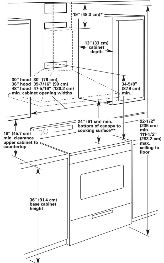
\* If the canopy hood is installed higher than 24" (61 cm) above the cooking surface, the middle bracket must be installed at the bottom point of the upper chimney sleeve.
