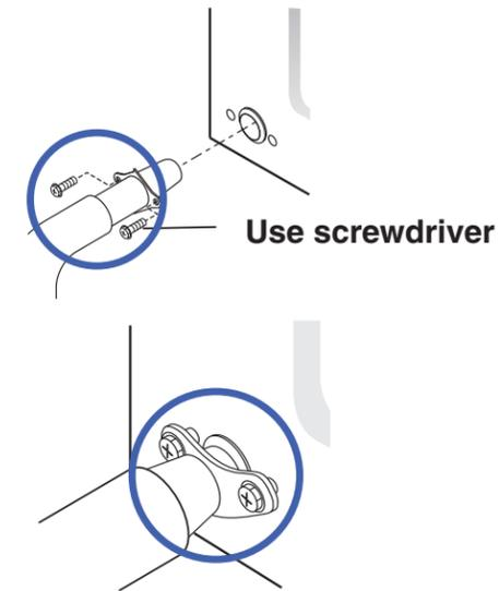
**Avoid a Repair!** Use clamps and screws for drain hose installation; without them leaks and flooding may occur
