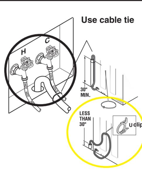
**Avoid a Repair!** Meet 30" drain hose height requirement. Less than 30" without U clip WILL NOT allow proper washer operation
