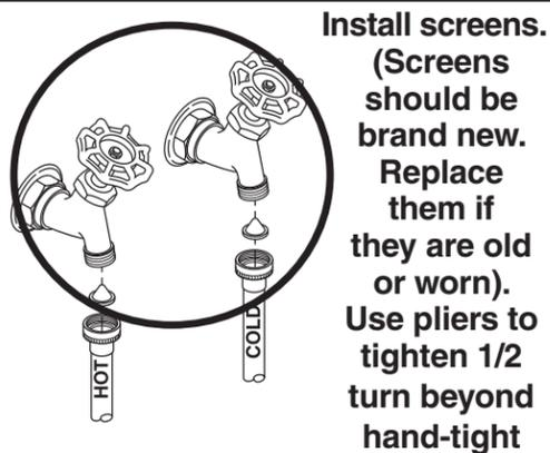
**Avoid a Repair!** Install screen washers; without them debris will clog the valve and flooding will occur
