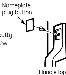
Remove the two screws holding the handle to the bottom of the door and remove the handle.
