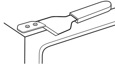
Reassemble the top hinge and shim on the left side, turning the screws just enough to hold the hinge in place.
