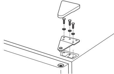
**NOTE:** On some models, when removing the door, watch for washer(s) between the center hinge and the bottom of the freezer door that may stick to the door. Do not lose.
