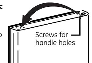
Carefully remove the button on the door by prying under the edge with a putty knife and transfer to the opposite side.
