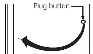
**Install handle:** Install the handle on the other side of the door.
