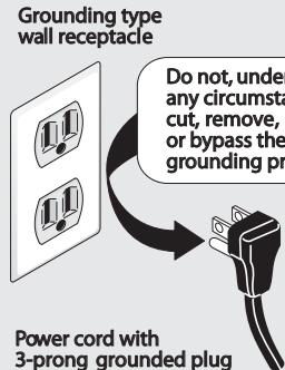
Avoid fire hazard or electrical shock. Do not use an adaptor plug or extension cord or remove grounding prong from electrical power cord. Failure to follow this warning can cause serious injury, fire or death.
