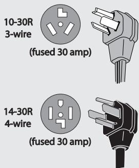
UL-approved service cord must be installed on electric dryers (not provided with unit except those manufactured for sale in Canada).
