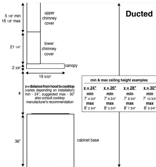
For ducted installations, the chimneys can be adjusted for ceilings between 7' 4 3/4" and 8' 9 3/4" depending on the distance between the bottom of the hood and the cooktop (**distance x in Ducted diagram**).
