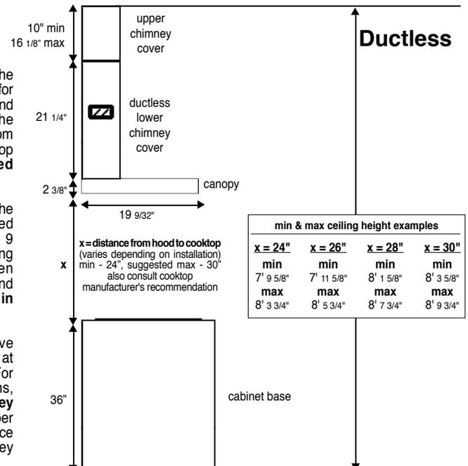
Note: If 24" or 30" High Backsplash is being installed, the distance between the bottom of the hood and the cooktop (**distance x in diagram**) is equal to the height of the Backsplash.
