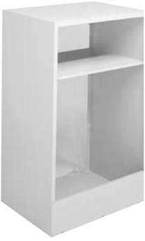
Since the unit itself does not install in the wall opening, the use of a plenum is necessary to contain and separate the outdoor air paths. The plenum must be able to hold water in the bottom without leaking into the wall cavity. It also must have a "splitter" to separate the outdoor air paths and prevent the discharge air from being drawn back into the unit.
