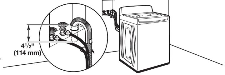
See requirements for floor standpipe drain system.
