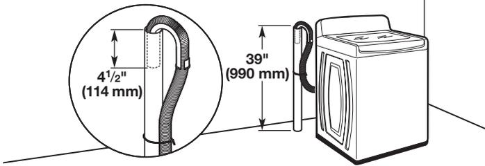
Minimum diameter for a standpipe drain: 2" (51 mm). Minimum carry-away capacity: 17 gal. (64 L) per minute. Top of standpipe must be at least 39" (990 mm) high; install no higher than 96" (2.4 m) from bottom of washer. If you must install higher than 96" (2.4 m), you will need a sump pump system.
