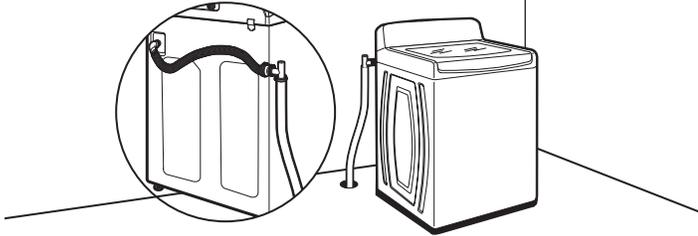
Floor drain system requires a Siphon Break Kit (Part Number 285834), 2 Connector Kits (Part Number 285835), and an Extension Drain Hose (Part Number 285863) that may be purchased separately. To order, please see toll-free phone numbers in your "Use and Care Guide." Minimum siphon break: 28" (710 mm) from bottom of washer. (Additional hoses may be needed.)
