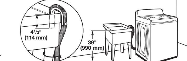
Minimum capacity: 20 gal. (76 L). Top of laundry tub must be at least 39" (990 mm) above floor; install no higher than 96" (2.4 m) from bottom of washer.
