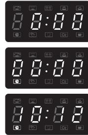
Note: In the process of clock setting, if the " STOP/CLEAR " button is pressed or if there is no operation within 1 minute, the oven will go back to the former setting automatically.
