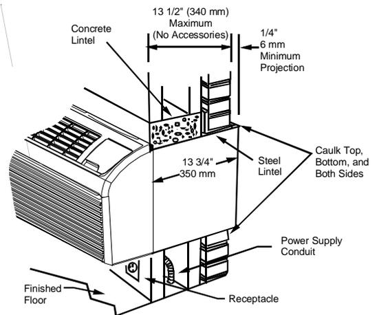
**Figure 6 - Block and Brick Veneer Installation**
