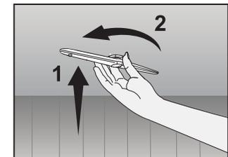
To replace the impeller, seat it into its slot, push slightly upwards and turn it counter clockwise until it is securely fitted. When the impeller is released, check if it rotates without any obstruction.
