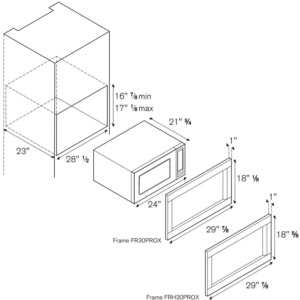
The minimum gap between the kitchen cabinet upper or lower panel and the appliance is  $\frac{1}{8}$ . This dimension must be added to the height listed in the drawings
