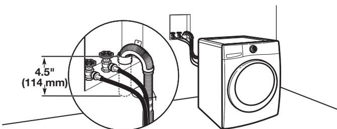
See requirements for floor standpipe drain system.
