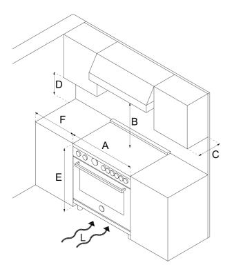
If installing toekick, verify that the sum of the cutout areas equal the recommended ventilation (L)
