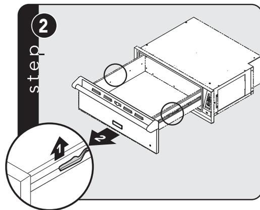
Slide finger along right and left side until you reach the hand latches (located approximately in the center of the rail). Pull up on the left side latch and press down on the right latch at the same time and pull out the drawer pan.
