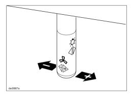
Use the joystick to select the desired time. Press it to the left for a shorter operating time, to the right for a longer operating time.
