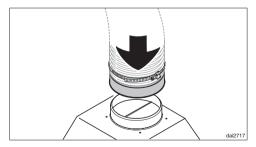
Place the exhaust hose onto the vent collar of the hood.
