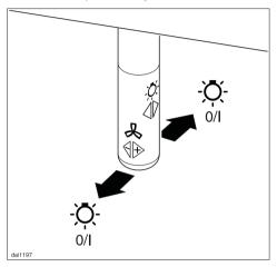
■ To turn the light on or off, press the joystick either once backwards or once forwards.
