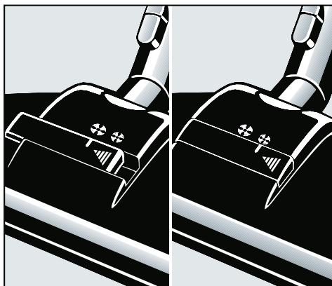
In all other situations the air adjustment slide should be closed, to benefit from the full suction power.
