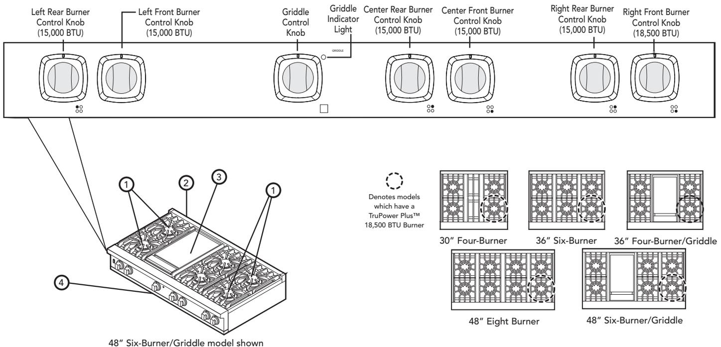
1. 15,000 BTU sealed burners/ Right Front 18,500 sealed burner
