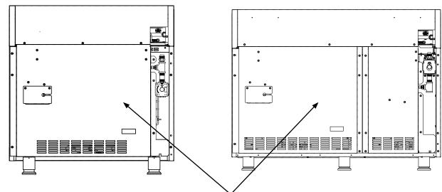
**NOTE:** VGR748 models have two regulators. Make sure both regulators are converted. To access second regulator, the island trim and small panel on the back must be removed
