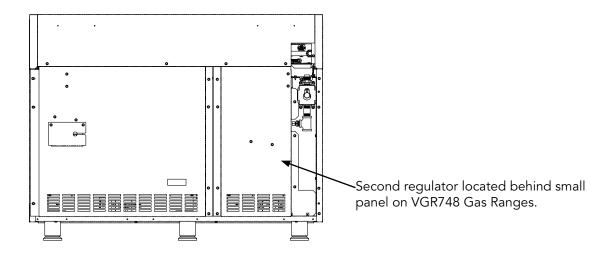
**IMPORTANT:** The infrared broiler orifice must be changed from rear of range before unit is installed. The island trim and rear panel must be removed to access infrared broiler.
