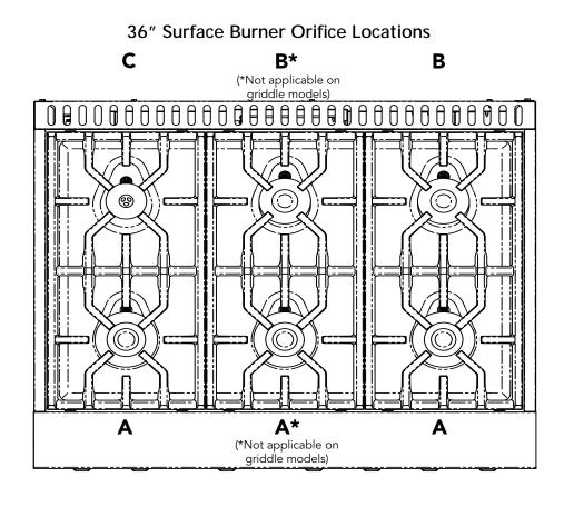
Burner A #44 (2.18 mm) Burner B #51 (1.70 mm) Burner C .048 (.1.22 mm)
