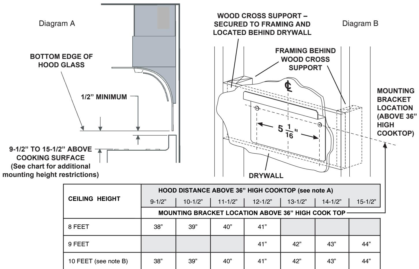
A. Minimum hood distance above cooktop must not be less than 9-1/2" (see Diagram B). Bottom of glass must clear the top of the range by at least 1/2". A maximum of 15-1/2" above the cooktop is highly recommended for best capture of cooking impurities. Distances over 15-1/2" above the cooktop are at the installer's and user's discretion - providing that ceiling height and flue length permit.
