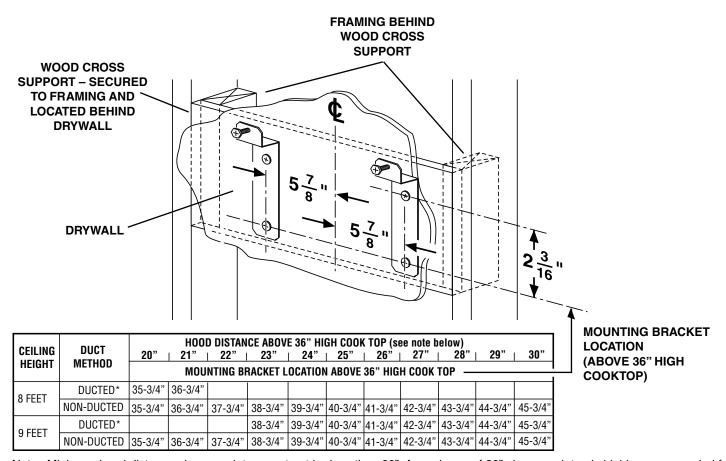
Note: Minimum hood distance above cook top must not be less than 20. A maximum of 30 above cook top is highly recommended for best capture of cooking impurities. Distances over 30 are at the installer and user's discretion; and if ceiling height and flue length permit.
