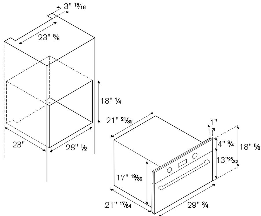
The minimum gap between the kitchen cabinet upper or lower panel and the appliance is 1/8. This dimension must be added to the height listed in the drawings
