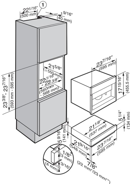
① Ventilation cut-out for installation in combination with a coffee machine
