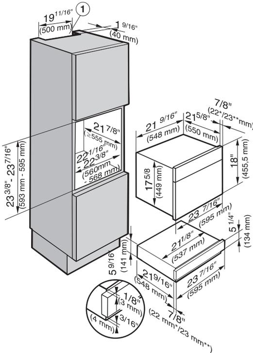
① Vent cut-out for when appliance is installed in combination with a combination steam cooker with oven
