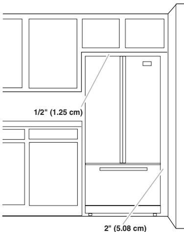
To ensure proper ventilation for your refrigerator, allow for a 1/2" (1.25 cm) of space on each side and at the top. Allow for a 1" (2.54 cm) space behind the refrigerator. If your refrigerator has an ice maker, allow extra space at the back for the water line connections. When installing your refrigerator next to a fixed wall, leave a 2" (5.08 cm) minimum space between the refrigerator and wall to allow the door to swing open.
