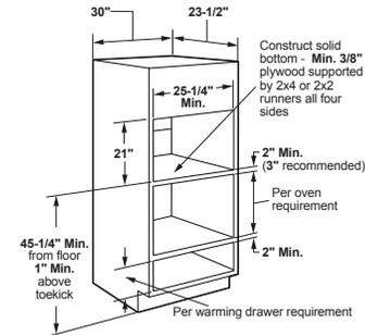
**NOTE:** Additional clearances between the cutouts may be required. Check to be sure the oven supports above the Warming Drawer location do not obstruct the required interior depth and height. See Warming Drawer installation instructions for details.
