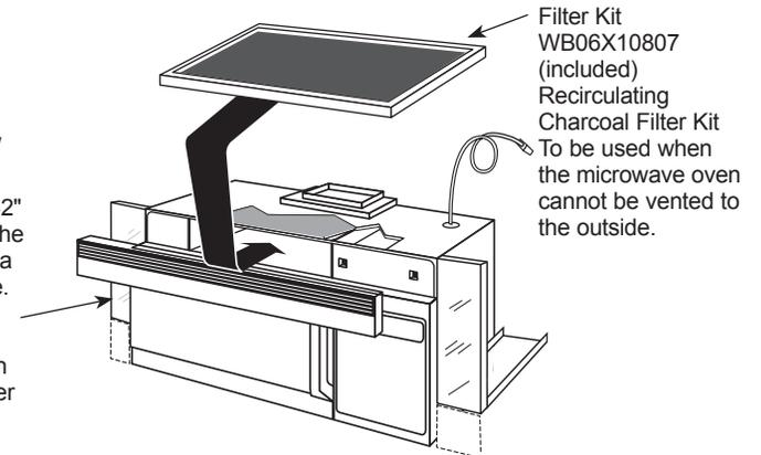
**Filter Kit WB06X10807 (included) Recirculating Charcoal Filter Kit**
